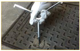
Configuration 1: with flat drill bit hook to clean and scrape.
